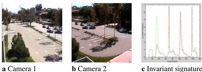
Fig. 11. Using invariant signatures for temporal registration. a Trajectory as observed from camera 1. b Trajectory as observed from camera 2. c Invariant signatures, green for the trajectory from camera 1 and red for the trajectory from camera 2
