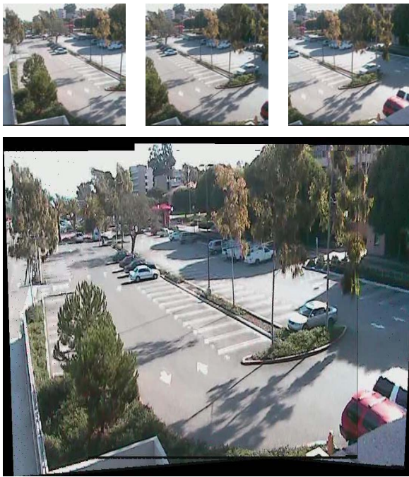
Fig. 10. Image mosaic. The upper row shows three input video frames of different spatial coverages. The bottom row shows the mosaic image constructed from the three input images that covers the whole parking lot
