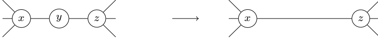
Fig. 5 Reduction Rule 2. Here the weight of new edge (x, z) is w((x, z)) = (w((x, y)) + w((y, z))) \bmod 2 .
