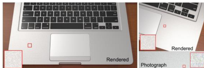
FIGURE 11. Left and top right: Rendering of a laptop with a point light and environment lighting using our wave optics method. Bottom right: A photograph of a MacBook (around 20 cm × 4 cm region) lit by a small LED light in a dark room. Our method is able to produce a colorful appearance that is perceptually similar to the photograph.
