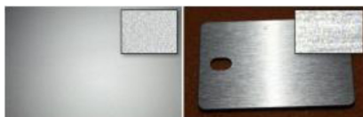
FIGURE 9. Real photos of the back of a laptop (left) and an aluminum patch (right), illuminated with only one LED light on a mobile phone. Even though we generally consider these objects white or colorless, the colors introduced by wave optics are always visible.
