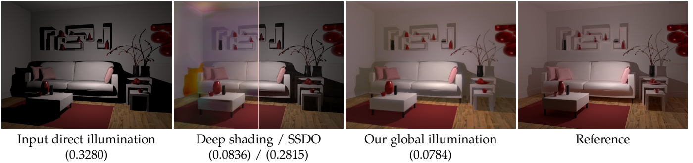
Fig. 1. Our method can predict high-quality global illumination with a resolution of 1024 \times 768 from direct illumination and auxiliary features such as normals and 3D positions. Our method runs at interactive framerates (45.3 FPS in this case) and generates much more plausible results compared with deep shading [1] and screen space directional occlusion [2]. The numbers above indicate the differences to the reference using the 1-SSIM metric.
