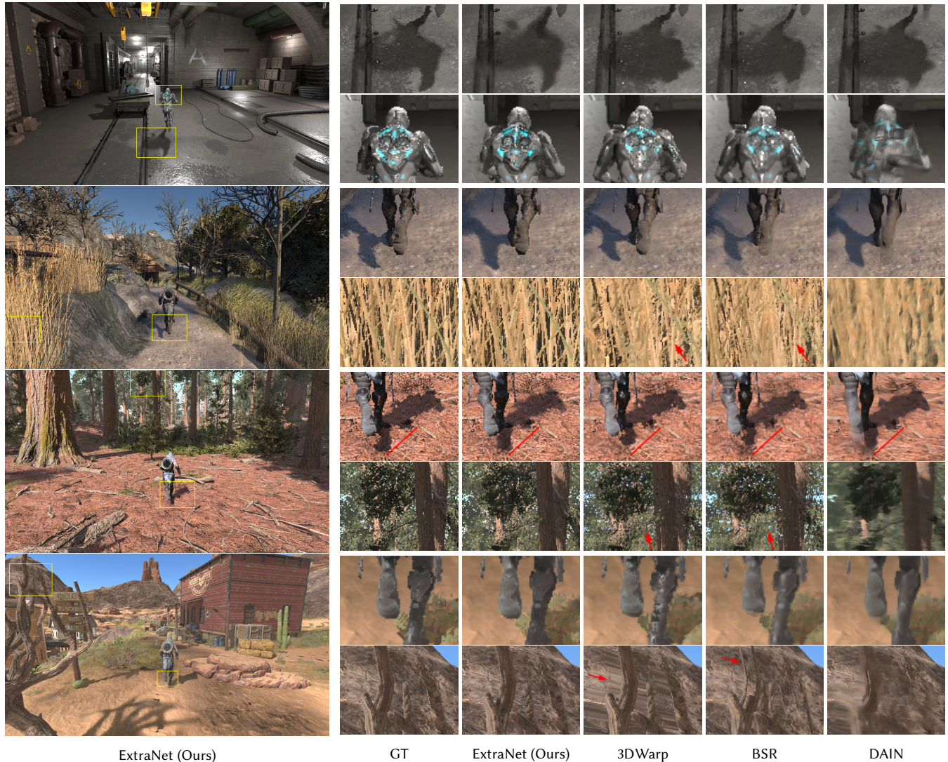
Fig. 13. Visual comparisons against three frame interpolation methods: 3DWarp [Mark et al. 1997], BSR [Yang et al. 2011], and DAIN [Bao et al. 2019]. Besides high latency, both 3DWarp and BSR may generate inconsistent moving objects and shadows, and will occasionally lose tiny structures. 3DWarp may also cause “rubber sheet” artifacts. DAIN generally achieves higher image quality, but is plagued with blurriness caused by large movements and absence of accurate motion vectors. Our deep learning-based frame extrapolation method avoids these problems and produces physically-plausible results that closely match the ground truth. In the closeups, red arrows highlight some artifacts that are not easily identified and red lines indicate the movements of shadows. See comparisons of animated sequences in the accompanying video.
