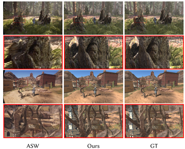
Fig. 16. Visual comparisons against Oculus' ASW technology [Oculus 2016]. Closeups in red boxes clearly show the artifacts generated by ASW due to incorrect optical flow.
