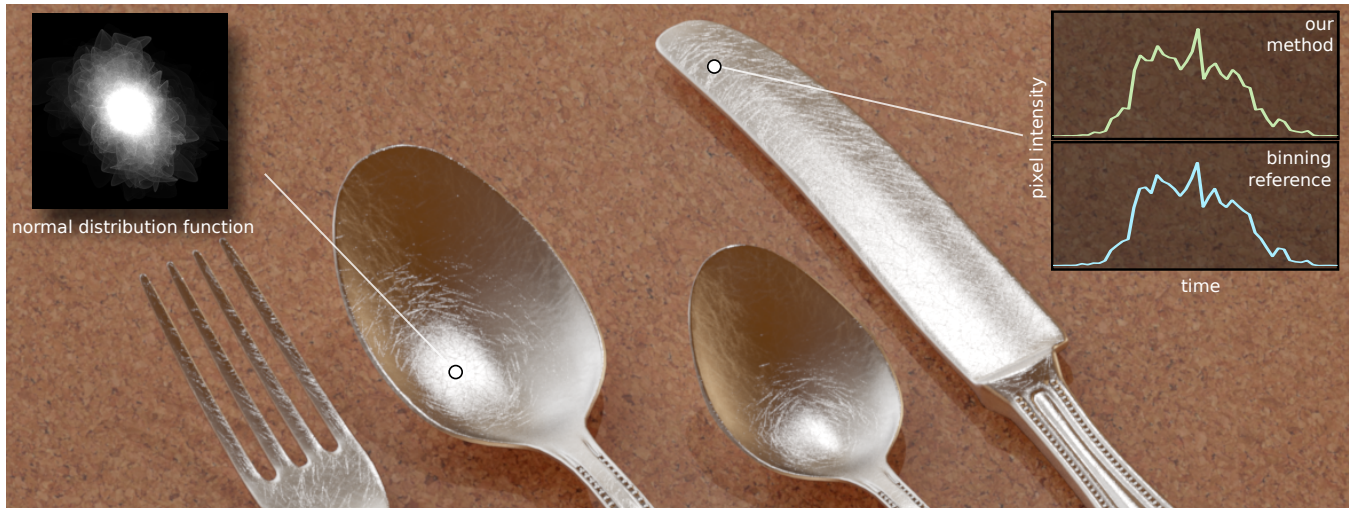
Figure 1: A rendering of specular objects with extremely low roughness (standard deviation of 0.001 radians) under point illumination. A high resolution normal map ( 2048^2 ) with scratches and small-scale noise makes rendering impractical with standard Monte Carlo direct illumination, since the highlights are tiny and easily missed by naive pixel sampling. Left inset: Our solution is based on the concept of a pixel normal distribution function (P-NDF), which can be highly complex. Our algorithm evaluates it exactly, instead of using simple approximations. Right inset: Our method delivers an accurate solution, even in a temporal sequence with a moving light.
