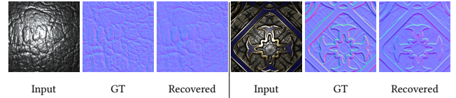
Fig. 3. Strong correlations exist between specular highlights and normal variation. In each group, we show the input image (Input), ground-truth normal (GT) and our recovered normal (Recovered).
