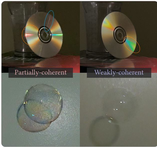
Fig. 2. Photographs of (top) a compact disk and (bottom) soap bubbles, illuminated by (left) a very small white LED source that admits a moderate degree of spatial coherence and (right) a larger array of lower intensity LEDs, which, together, produce weakly-coherent radiation. Both sources have similar spectrum. The diffraction grating on the compact disk gives rise to primary diffraction lobes (outlined in orange). In addition, secondary diffraction lobes (outlined in cyan) appear as well under illumination by a more coherent source. The soap bubbles are made of an identical mixture and are akin in chemical composition. Nevertheless, the thin-film interference effects are clearly visible on the left and virtually not at all on the right, indicating the important role optical coherence plays. See our supplemental material where we include videos of these soap bubbles.
