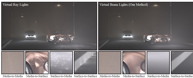
Fig. 7 Indirect illumination on surfaces and in the medium. Progressive virtual ray beams (right) significantly reduce singularity artifacts compared to the virtual ray lights method (left). Progressive render effectively eliminates singularities in four indirect light transport paths (bottom) using novel importance schemes and a new lighting primitive compatible. Figure reproduced from [56].
