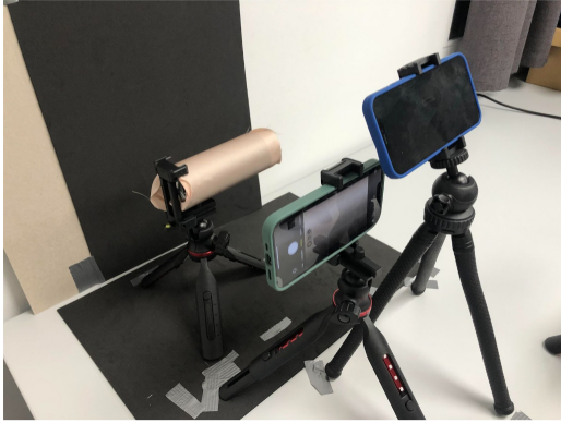
Figure 4: Measurement setup for cloth appearance capture. The cloth sample is wrapped onto a cylinder, and photographed from a cellphone with known camera intrinsics. The scene is illuminated by the flash light of a second cellphone with known position.
