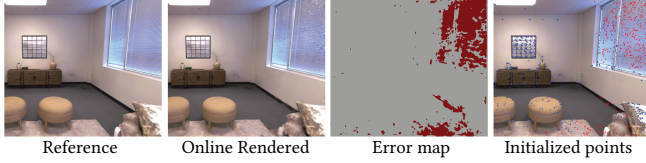
Fig. 3. A visualization of pixels used for initialization. In the error map, red regions indicate high-error areas. In the right-most image, red points represent pixels used for error compensation, while blue points correspond to pixels in geometry- or texture-complex regions.
