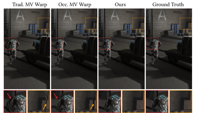
Figure 4: Comparison of different warping methods. Our method generates better warping results without ghosting artifact while both traditional warping and occlusion motion vectors generate incorrect shading in the disoccluded areas.
