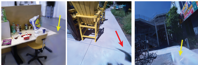
Fig. 4. Failure cases of our method. Left : Misaligned ghosting artifacts caused by severely inaccurate and shifted tracked camera poses. Middle : Overfitting artifacts arising in the presence of dynamic objects within the scene. Right : Low-quality reconstruction in regions that are poorly observed.
