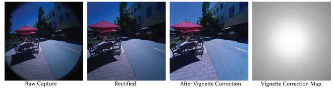
Fig. 1. Illustration of Aria captured images pre-processing. The raw captured image's resolution is 2880 \times 2880 .
