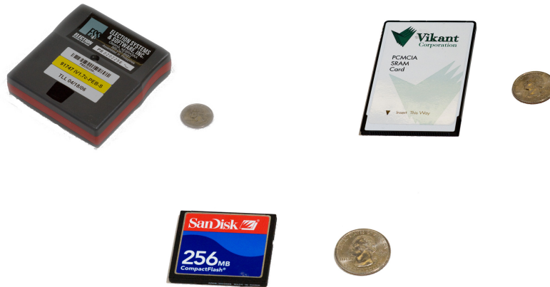
Fig. 3. The Data Transport Devices used in the ES&S voting system. The reference coin is a US quarter, whose diameter is 24.26 millimeters.
