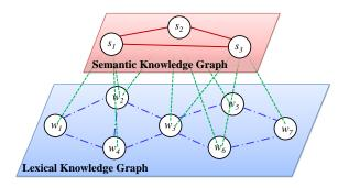
Figure 3: A simplified example of the two knowledge graphs, where a slot candidate  $s_i$  is represented as a node in a semantic knowledge graph and a word  $w_j$  is represented as a node in a lexical knowledge graph.
