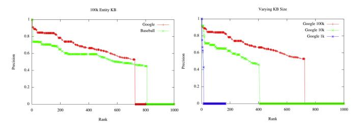
Figure 5: Performance on completing subsets of the NELL KB. Left, interpolated precision vs rank for two KBs with 100k entities; right; comparison on three KBs of different sizes based on the seed "Google".
