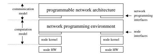
Figure 2: Generalized Model for Programmable Networks
