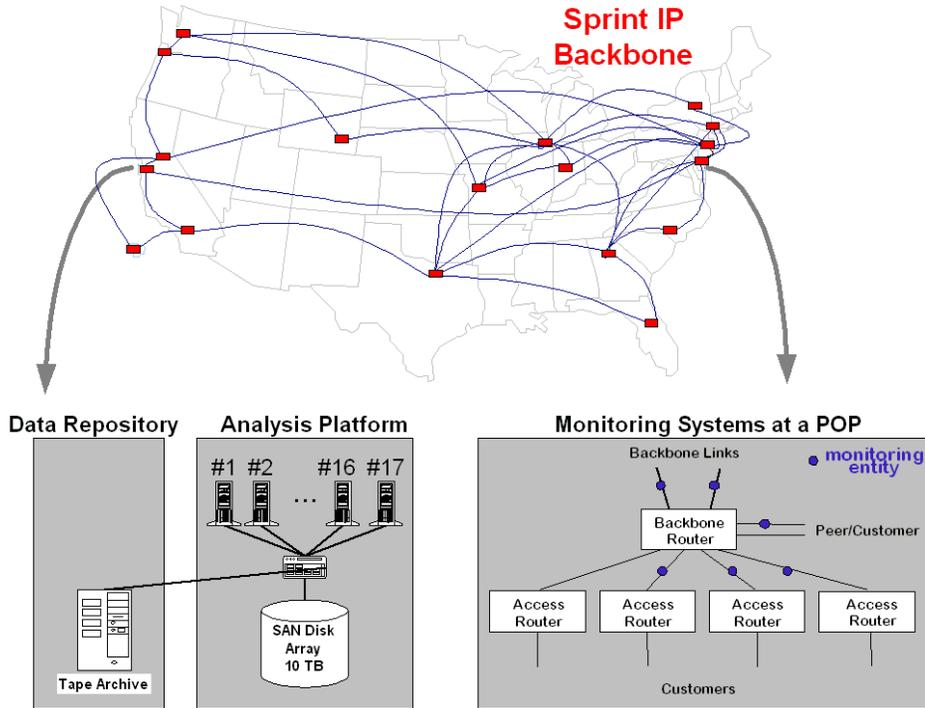
Fig. 1. The IPMON system in the Sprint IP backbone
