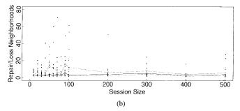
Fig. 15. Local recovery with two-step repairs in bounded-degree trees with 1000 nodes, thresholds of one.
