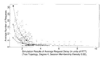
Fig. 8. Tradeoff between delay and duplicates for sparse sessions in a tree topology.
