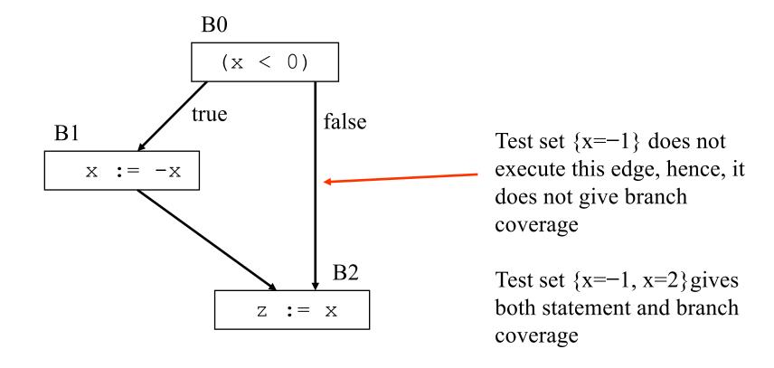
Select a test set T such that by executing program P for each test case d in T, all paths leading from the initial to the final node of P's control flow graph are traversed
