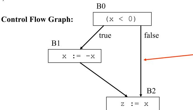
Test set {x=-1} does not execute this edge, hence, it does not give branch coverage
