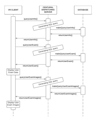
Figure 7: VR application query sequencing diagram
