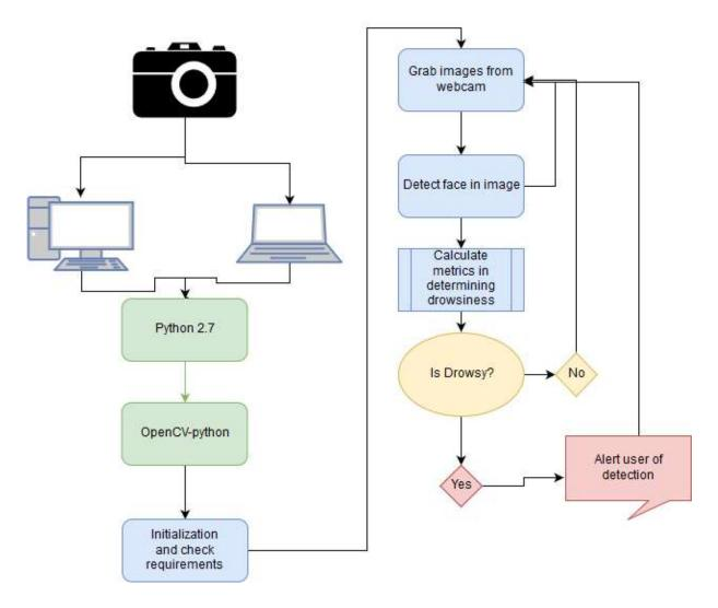
A user will run the executable program which will then check to make sure correct version of Python and OpenCV are installed. There will be a button to press start. Once start is pressed, the program will start all functionality and detect whether the user is drowsy. The button will then say stop which can be pressed to halt the program.
