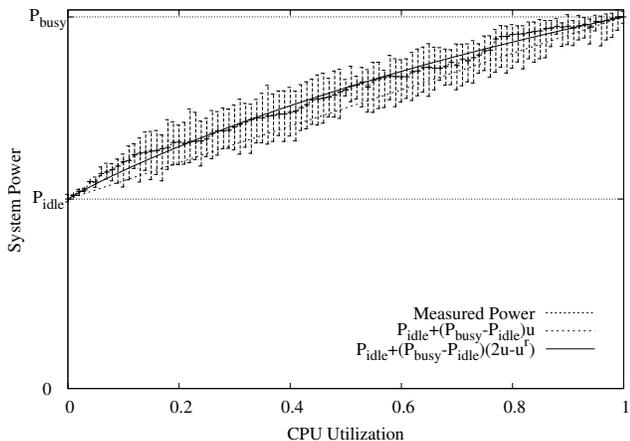
Figure 2: Model fitting at the machine level
