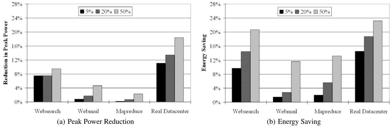
Figure 10: Impact of CPU DVS at Datacenter Level
