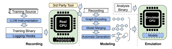
Figure 2: High-level design of CONWARE: logging hooks are inserted into the compiled binary, the binary is run on real hardware to extract a detailed log, these logs are then converted into concise state-machine representations, and then both the uninstrumented binary and the models are run on emulated hardware, enabling detailed, scalable analyses.
