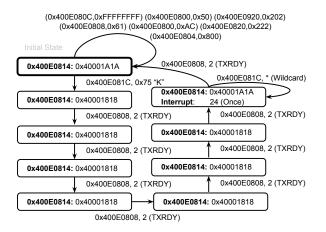
Figure 5: An  $\omega$ -automata for a UART peripheral generated from a recording that prints "Knock!\r\n" repeatedly. The initial state will accept all configuration parameters, once a "K" is written, the peripheral becomes BUSY until the READY state is reached and interrupts are thrown.
