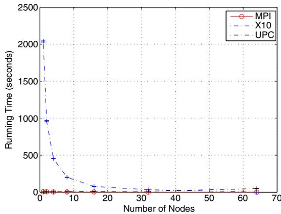
**Fig. 7** Average running time for the Thread Ring code utilizing MPI, X10, and UPC over varying numbers of nodes. These timings only include execution times reported by each language’s timing constructs
