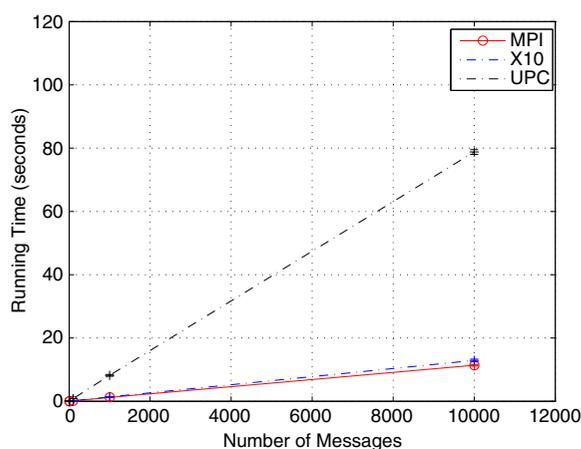
**Fig. 9** Average running time for the Thread Ring code utilizing MPI, X10, and UPC over varying numbers of messages. These timings only include execution times as reported by each language's timing constructs
