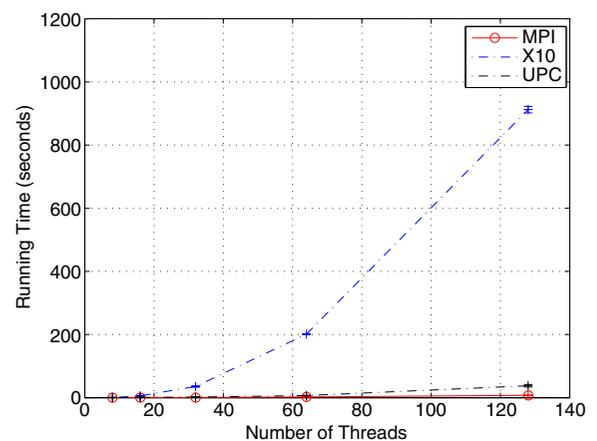
**Fig. 8** Average running time for the Thread Ring code utilizing MPI, X10, and UPC over varying numbers of threads. These timings only include execution times as reported by each language’s timing constructs
