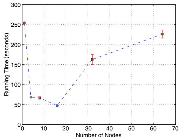
**Fig. 4** Average running time for the Power Method code utilizing MPI over varying numbers of nodes. These timings include running time as reported by *MPI\_Wtime* and do not include NFS and MPI startup and shutdown times
