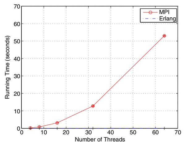
**Fig. 10** Average running time for the single node Thread Ring code utilizing MPI and Erlang over varying numbers of threads. These timings only include execution times as reported by each language's timing constructs
