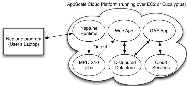
acquires nodes to run the code over, configures them for use, and executes the code, storing the output for later retrieval. In the case of a data input or output job, the Neptune runtime stores or retrieves the data via the datastore.
