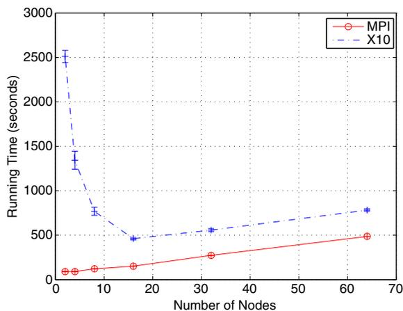
**Fig. 5** Average running time for the n-queens code utilizing MPI and X10 over varying numbers of nodes. These timings include running time as reported by *MPI\_Wtime* and *System.nanoTime*, respectively. These times do not include NFS and MPI startup and shutdown times
