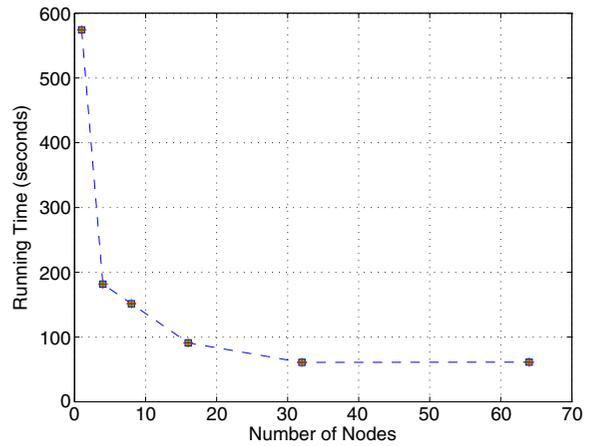
**Fig. 12** Average running time for the dwSSA code over varying numbers of nodes. As the code used here does not have a distributed runtime, timings here include the time that AppScale takes to distribute work to each node and merge the individual results
