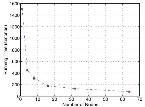
**Fig. 6** Average running time for WordCount utilizing MapReduce over varying numbers of nodes. These timings include Hadoop MapReduce run times and do not include Hadoop startup or shutdown times
