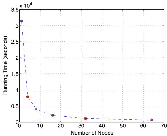
**Fig. 11** Average running time for the DFSP code over varying numbers of nodes. As the code used here does not have a distributed runtime, timings here include the time that AppScale takes to distribute work to each node and merge the individual results
