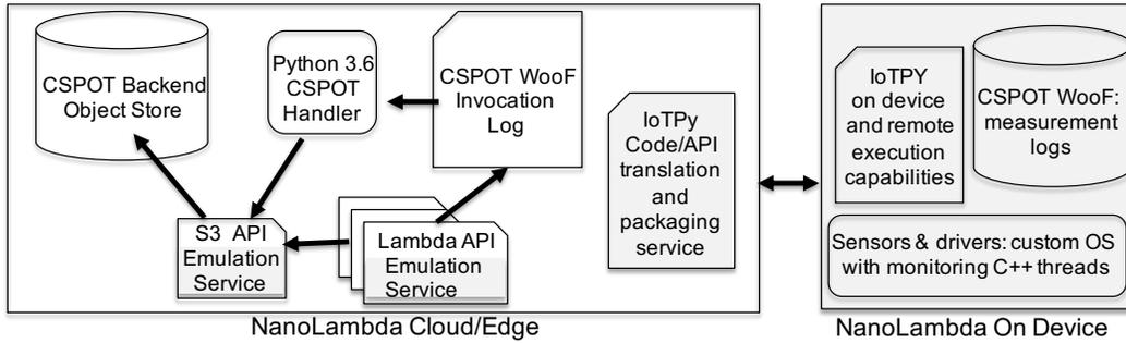
Fig. 1. Service diagram outlining the interactions of the *NanoLambda* components that deliver FaaS for IoT. Shaded components are those added to *CSPOT* by *NanoLambda*. *NanoLambda Cloud/Edge* runs on Linux hosts in the cloud or at the edge; *NanoLambda On Device* runs on microcontrollers and non-Linux systems.
