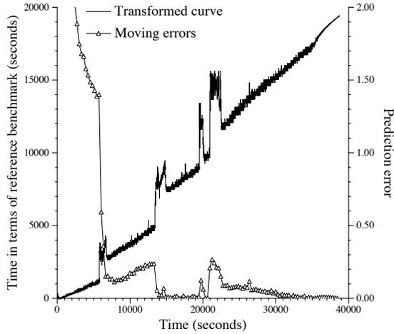
Figure 10: Transformed voltage curve and moving errors for real.load.4. The left  $y$ -axis is the transformed voltage in terms of time for reference curve. The right one shows the value of errors. We set the maximum to be 200% and those larger errors in the early period of time are not shown.
