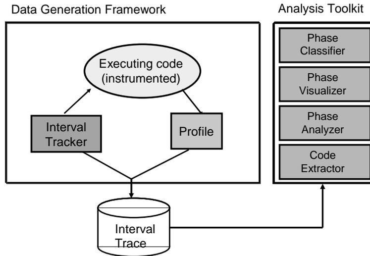
Figure 1: JVM framework and toolkit for the analysis of phased behavior in Java programs.
