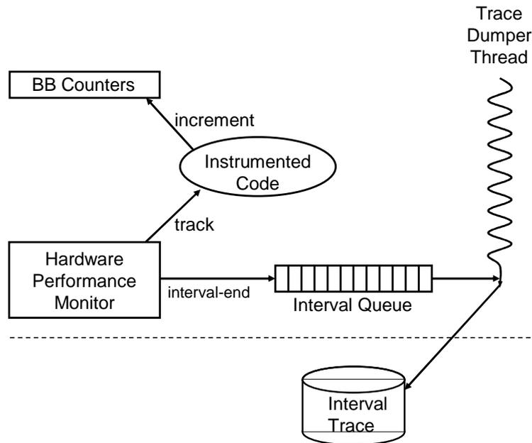
Figure 2: Architecture of the data generation framework. The instrumented application updates counters for the current snapshot (profile) interval in an interval queue. When the hardware performance monitors (HPMs) indicate that the interval granularity has been reached, a background dumper thread is signalled. The dumper thread expels all past snapshots to an interval trace on disk. The HPMs collect hardware data on a per-thread data; we monitor only application threads.
