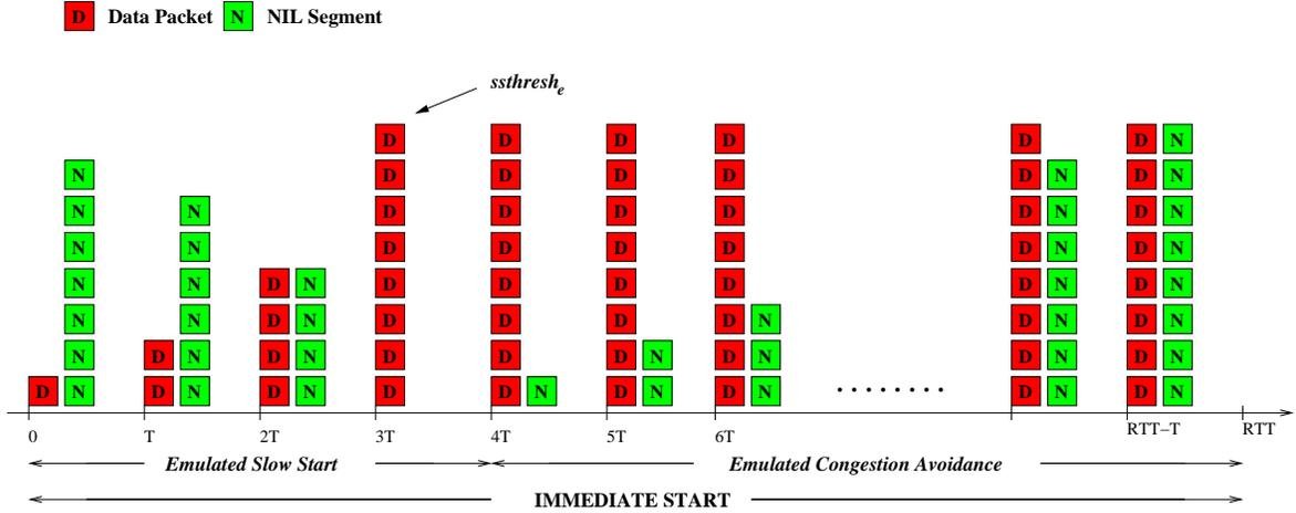
Fig. 3. An example illustration of time framing mechanism in the Immediate Start phase for  $ssthresh_e = 8$ .
