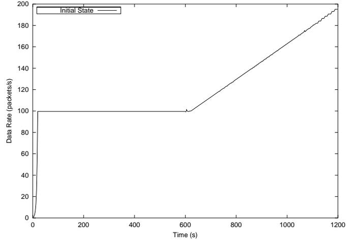
Fig. 9. Transmission rate change in the Initial State of TCP-Planet source for  $RTT = 600$  seconds.
