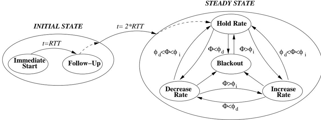
Fig. 2. TCP-Planet protocol operation state diagram including substates and the state transitions based on congestion control decision mechanism.
