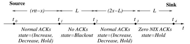
Fig. 7. Blackout condition observed from TCP-Planet source for  $L < 2x$ .
