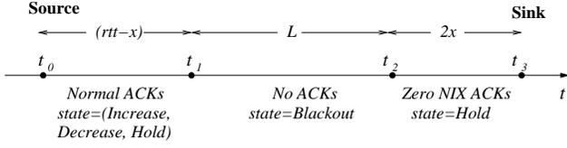
Fig. 8. Blackout condition observed from TCP-Planet source for  $L \geq 2x$ .
