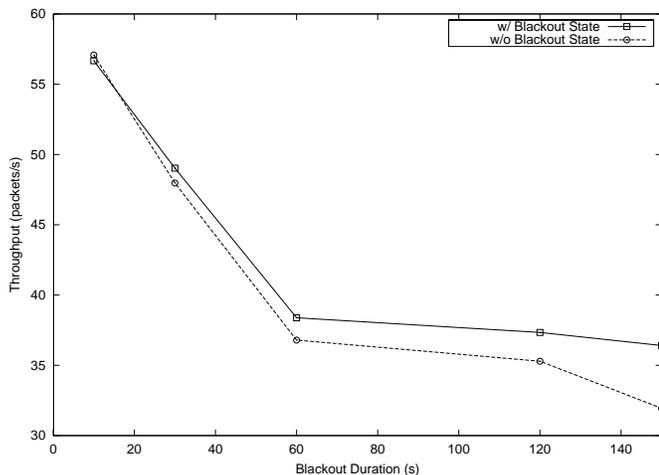
Fig. 14. Throughput for changing blackout duration with  $RTT = 120$  seconds and  $p = 10^{-5}$ .
