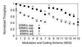
(d) Channel leakage from a neighboring 40MHz transmission
