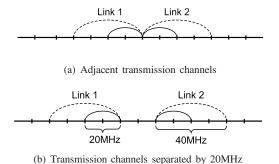
Fig. 4. Separation cases between non-overlapping channels: (a) adjacent channels, and (b) 20MHz channel width apart.
