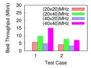
Fig. 6. Best throughput for a link (location 1 in Fig. 5) suffering from co-channel interference. In Test Case 1, the overlapping transmitter has good link quality to its receiver and operates at MCS 10. In Test Case 2, the overlapping transmitter has poor link quality to its receiver, and thus operates at MCS 0.
