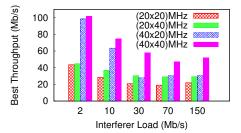
Fig. 8. Best throughput for a link suffering from cochannel interference with varying interferer load. We define the legend: (transmitter's bandwidth × interferer bandwidth)MHz.
