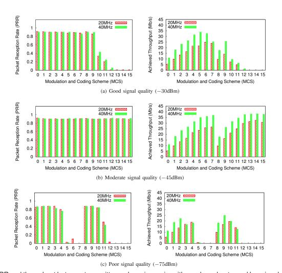
Fig. 3. PRR and throughput between transmitter and receiver pairs with good, moderate, and low signal qualities.
