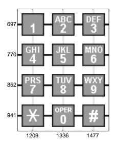
Figure 8.1. Telephone keypad.
