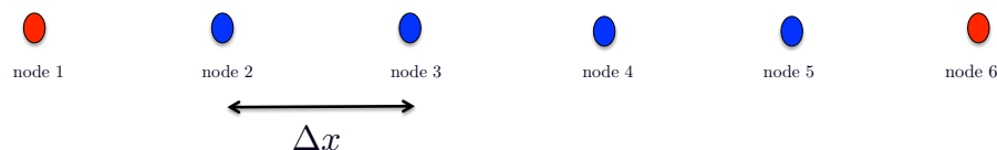
Figure 1: Discretization of a one dimensional domain with m = 6 nodes. The solution u at the red nodes will be given the value of the boundary conditions through the function BC , while at the blue nodes the solution will be approximated using (3).
