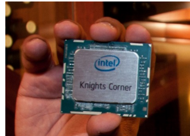
61-processor Intel Xeon Phi: 1.0 TFLOPS
