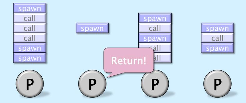
Each worker (processor) maintains a *work deque* of ready strands, and it manipulates the bottom of the deque like a stack
