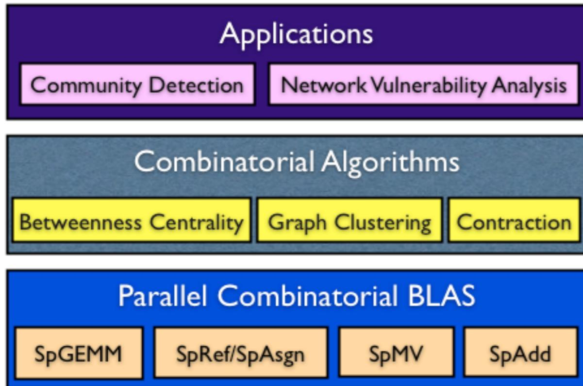
A typical software stack for an application enabled with the Combinatorial BLAS
