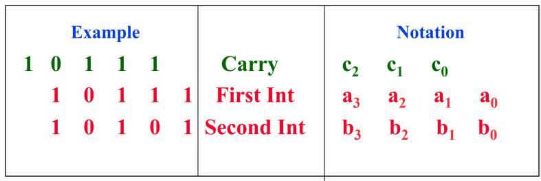
$c_{-1} = 0$ for i = 0 : n-1  $s_i = a_i + b_i + c_{i-1}$  $c_i = a_i b_i + c_{i-1} (a_i + b_i)$ end
