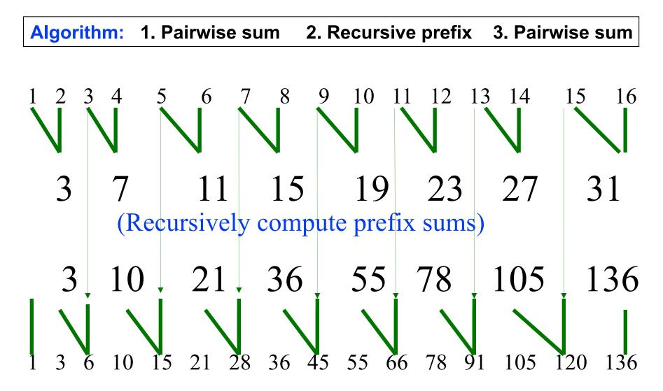
Parallel prefix cost: Work and Span
