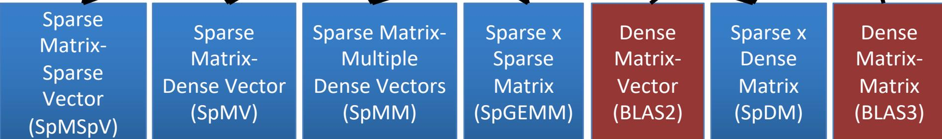
Graph/Sparse/Dense BLAS functions (increasing arithmetic intensity) →
