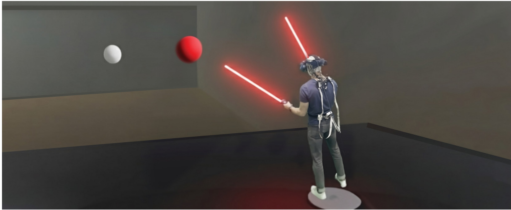
Figure 1: A participant is shown superimposed into a virtual environment, standing on a platform wielding a pair of virtual sabers anchored to HTC Vive Controllers. They are required to strike incoming spheres using either saber while their brain activity is recorded at the scalp using electroencephalography (EEG).
