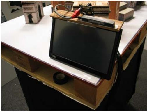
Figure 1: The display device used for both experiments. The device uses a MIMO iMO 10 inch USB display, a Point Grey FireFly camera, and an IS900 Headtrax device.
