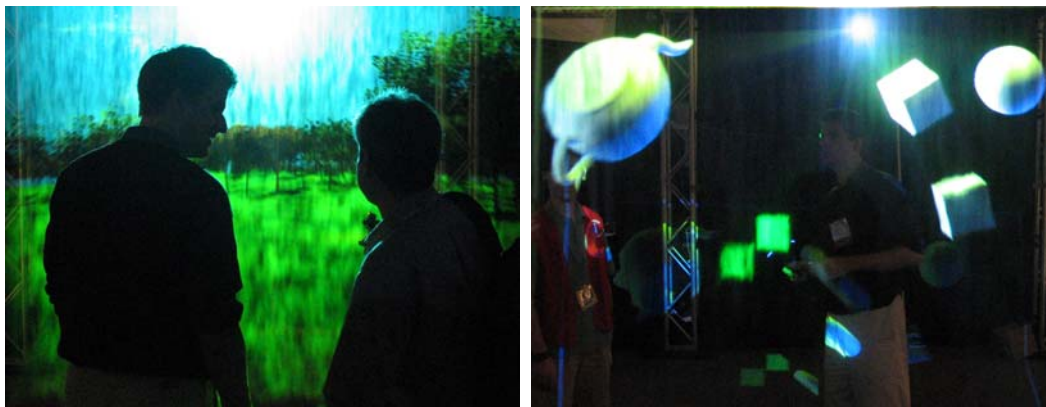
Figure 1: FogScreen can create fully opaque or very translucent high-quality images in mid-air. It can provide high visual detail.
