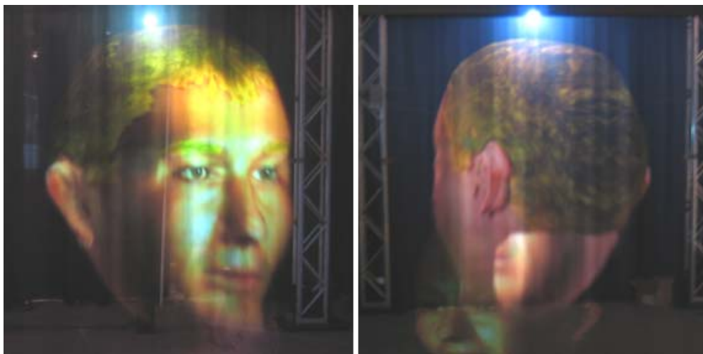
Figure 5: The FogScreen's support for dual-sided projection allows two independent images to be projected on each side of the screen, such that the opposite sides of a 3D object can be rendered on the screen for a pseudo-3D effect. Left: front view. Right: rear view (as the head model's geometry is open at the neck, the front side of it is visible there).
