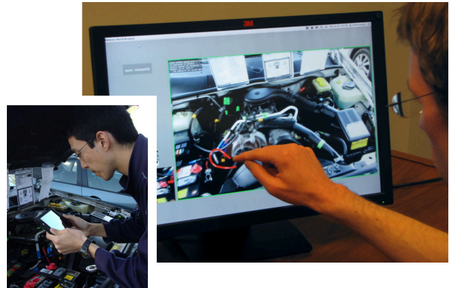
Figure 1: A remote user points out an element in the environment (here: a car’s engine bay) by drawing an outline around it. The annotation is world-stabilized and displayed in augmented reality to the local user (bottom left), who is holding a tablet.
