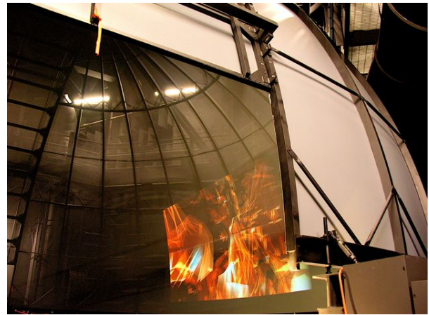
Figure 6: Testing the Allosphere projection with a single 2K active stereo projector and brain imaging data
