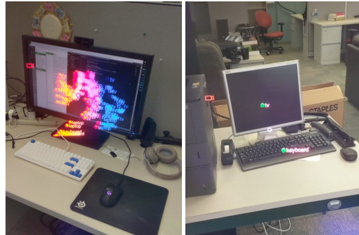
Figure 1: Left: Raw points returned from object recognition as projected into 3D space, accumulated over several frames. This shows the variance in predicted positions and false positive label predictions. Right: Scene correctly labeled after object registration.
