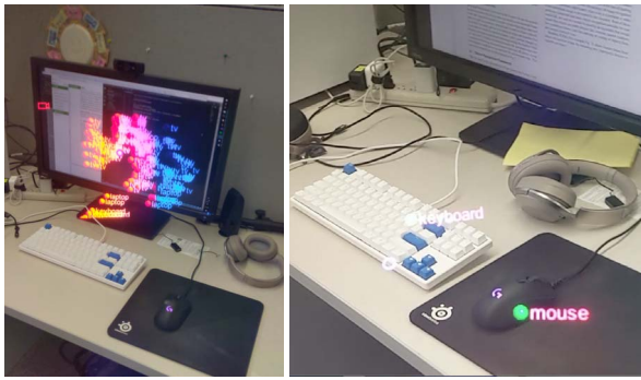
Figure 3: Left: Raw points returned from object recognition as projected into 3D space, accumulated over several frames. This shows the variance in predicted positions and false positive label predictions. Right: Scene correctly labeled with object-permanent labels.
