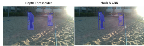
Figure 2: An example image where Mask R-CNN fails to mask the person occluded in the background while the depth thresholder does.
