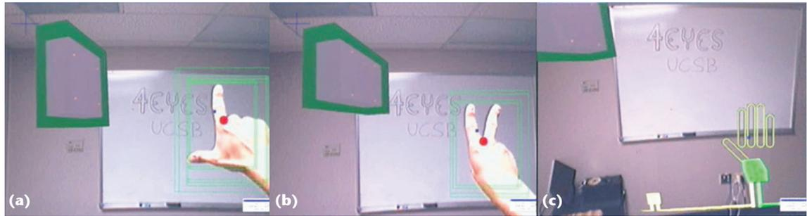
**7 Resizing an object with gestures.** (a) The user's hand in the lock posture from which hand location changes rescale the virtual object (the gray box with a green selection frame around it). (b) The user performs the release posture, which decouples hand movements and object scale again. (c) The placement of the virtual object in the upper left corner and representations for power and networking equipment near the floor.
