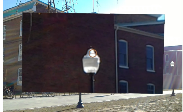
Figure 8: User’s view of ImageRefinement in the HoloLens. The user adjusts the ray by moving the crosshair in the 2D image.
