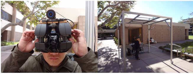
Fig. 3. The display system used for this experiment consisted of: an NVis SX111 HMD, a Pointgrey USB3 Flea camera, and an InterSense IS900 tracking system. The image on the left shows the HMD setup with the camera and the image on the right shows the custom tracking frame built for the outdoor condition. For the simulated conditions with the low, mid, and high models, the experiment was conducted indoors with the same display and tracking systems.
