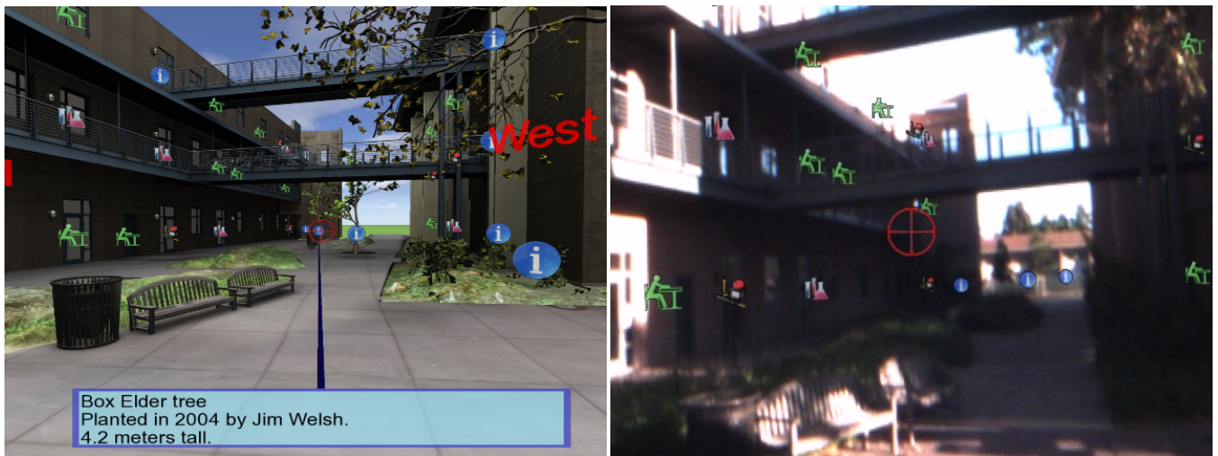
Fig. 2. The high-fidelity model and the real environment, both with virtual annotations. There are four different types of annotations: The blue icon with the “i” represents miscellaneous information. The green icon that looks like a student at a desk represents classroom information. The icon with beakers indicates lab information. And the pen and ink icon indicates information about an office. The real environment here was captured at a lower resolution, but the lighting artifacts are accurately represented.
