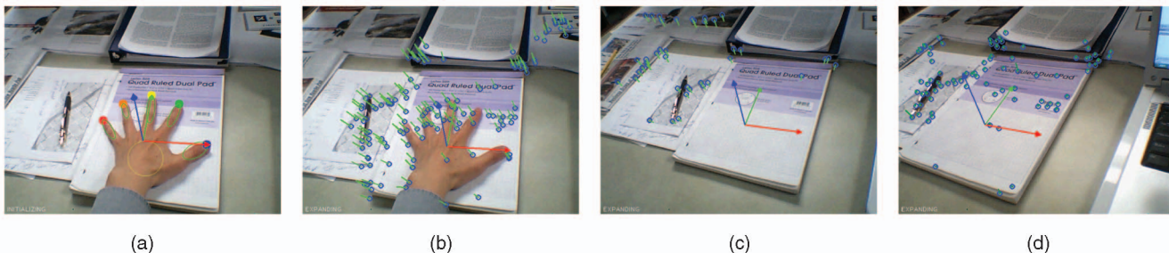
Fig. 3. Establishing a coordinate system using Handy AR (a), propagating it to the scene as we detect scene features (b). After moving the hand out of the scene (c), new features are detected from the area that the hand occluded (d).
