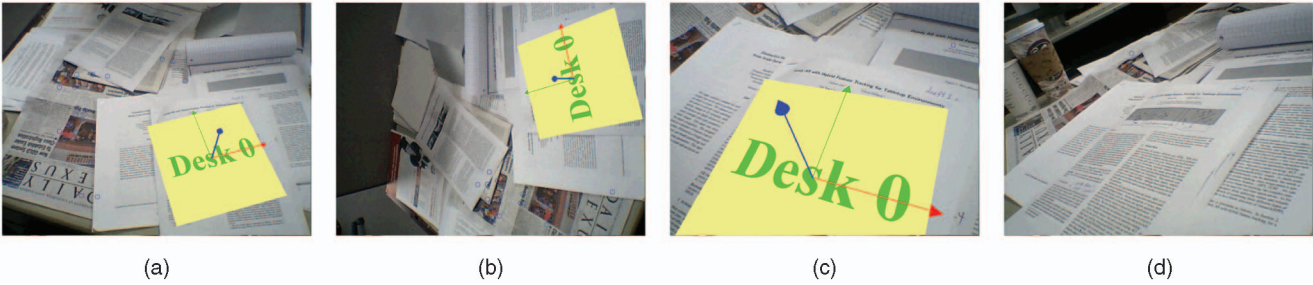
Fig. 13. (a), (b), (c) Various angles of camera pose, estimated from the features in the scene. (d) Exceeding a certain viewing angle, SIFT features are no longer matched.
