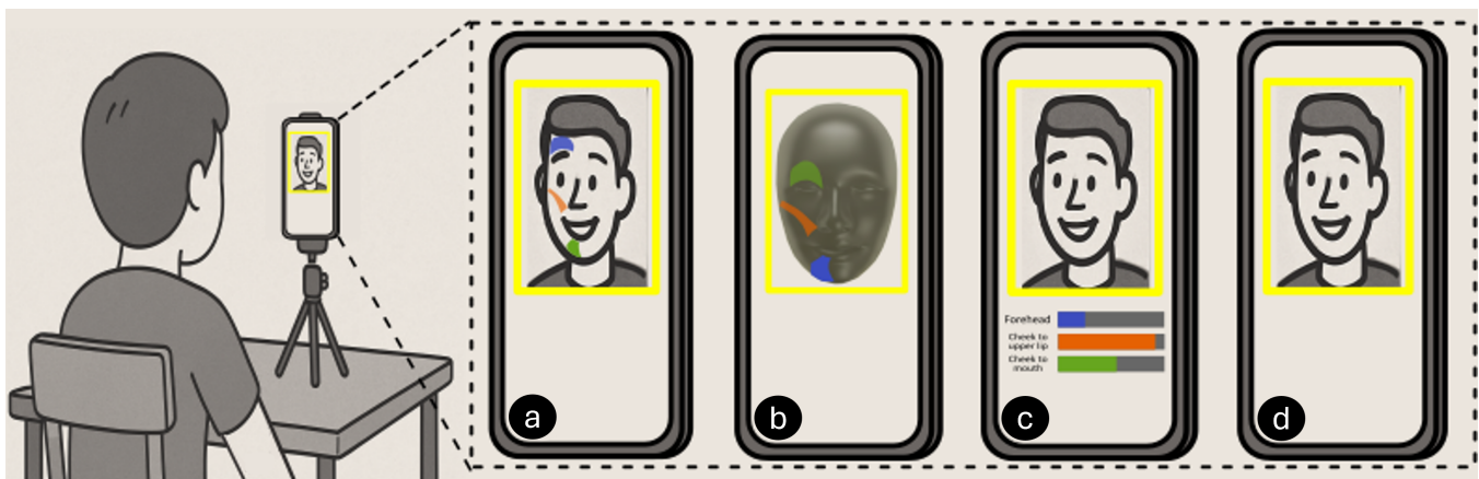
Figure 1: A participant engages in AR-guided facial exercises, receiving real-time feedback designed to improve muscle movement patterns. We evaluate three AR-based feedback conditions, (a) embedded ARSelfie with feedback overlaid on the user's own face, (b) proxy-embedded Mannequin with feedback on a 3D avatar, (c) situated BarChart with feedback conveyed through bars located below the user's face and (d) a no-feedback Baseline condition where the user can see themselves. We assessed how the spatial placement of feedback affects user performance, experience and cognitive load. [Portions of this image were generated using AI.]
